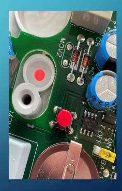
On the Ei428 Relay press the House Code button (Red) as per picture above when the LED comes on let go of the button. The LED will now flash.
